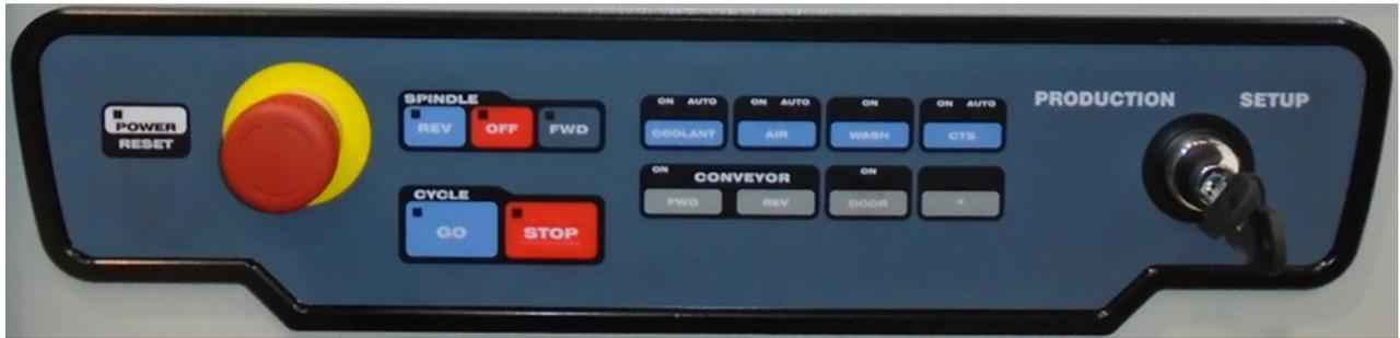
**POWER RESET:** This button is used to reset the machine from a hardware E-stop condition or NC Not Ready state.. It will need to be pressed at first power up and any time the control gets into a critical fault condition. For example, if the user presses the Emergency Stop button.
